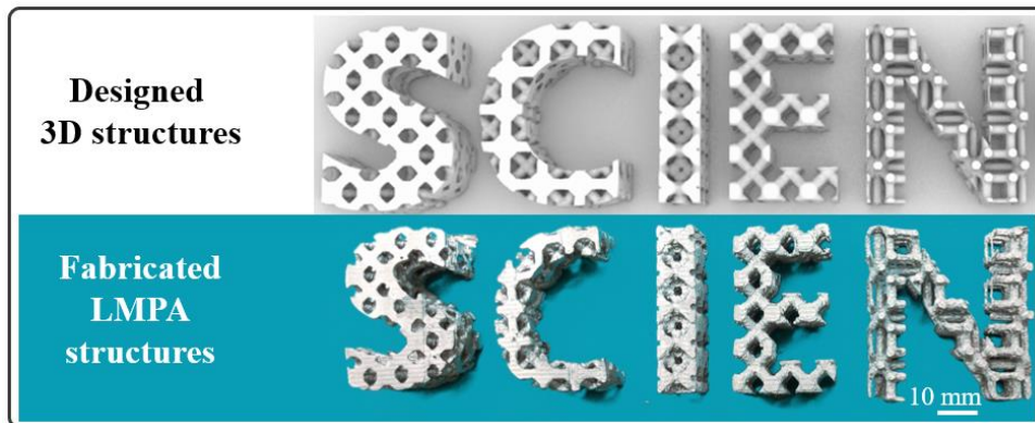
Fig. 6 Demonstration of printed complex pure LMPA parts.
