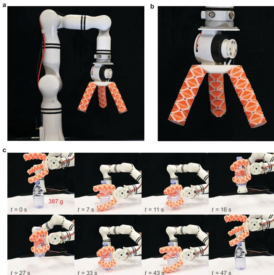
**FIG. 9.** Assembly and grasping performance of the origami gripper. (a) Demonstration of the origami gripper in action. (b) Physical prototype of the origami gripper. (c) Grasping experiment of the origami gripper.
