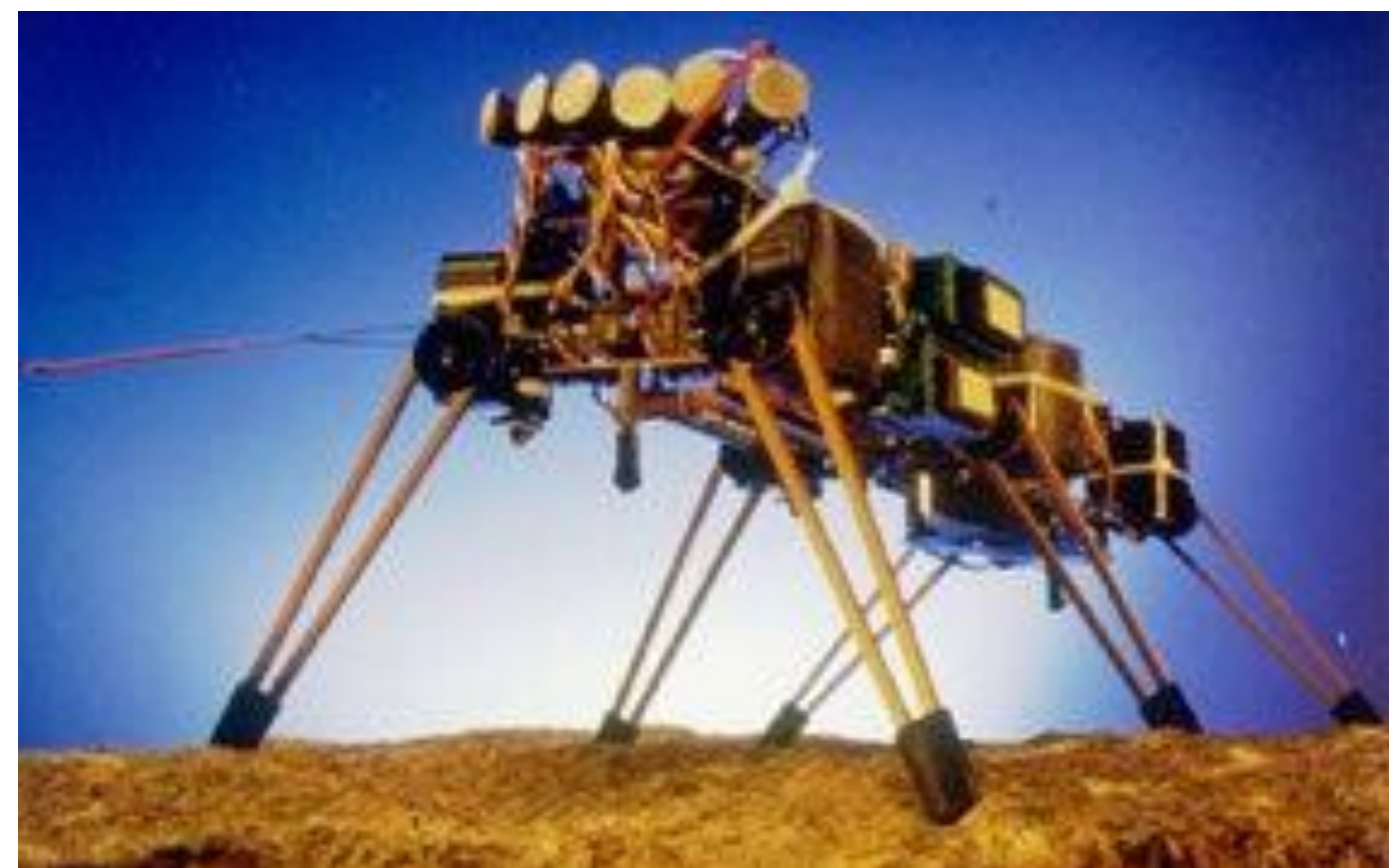
Genghis robot: a six legged hexapod robot
