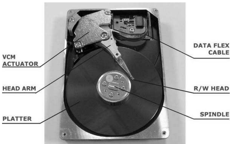
Figure 9.1. An HDD with a VCM actuator
