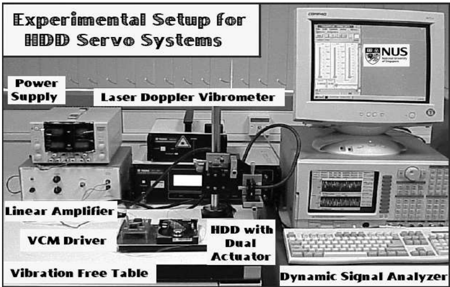
Figure 1.7. Implementation setup for HDD servo systems
