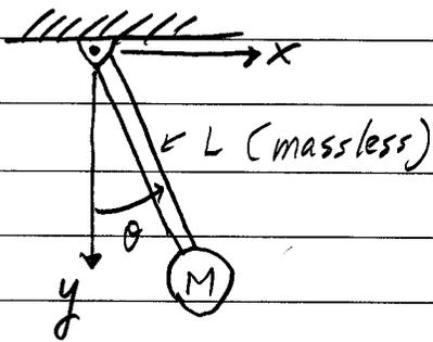
the planar motion of a pendulum
