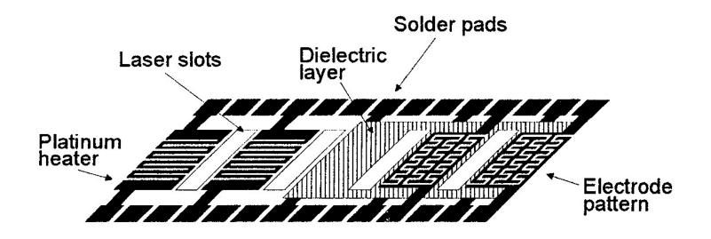
An example of an array of chemiresistors fabricated using thick-film techniques. The slots are cut by a laser and help to isolate each sensor site from its neighbors
