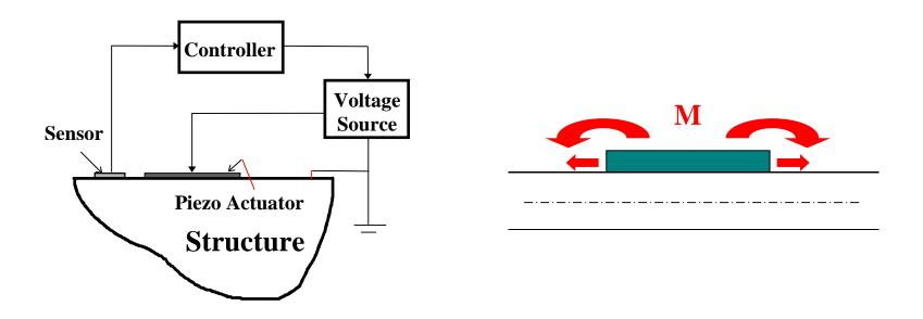
Piezoelectric materials have shown to be effective active structural control elements:
