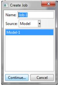
In the Edit Job window, select OK, as we will be using default values for this example. Now under Analysis>Jobs, right-click on Job-1 and select Submit. After a few seconds, "Job Job-1 completed successfully" will appear in the terminal at the bottom of the window. We are now ready to view the results.
