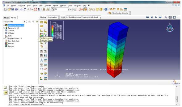
Now say we want to plot the axial component of stress along the bottom face of the bar. At the top of the screen, under the Tools menu, select Path>Create Path. Select
