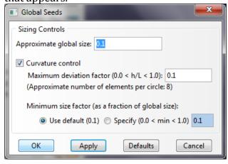
The seed-points for the mesh should appear on the part. Next click the Mesh Part Instance button in the toolbar (directly below Seed Part Instance button). Press Enter. The part should now appear meshed.
