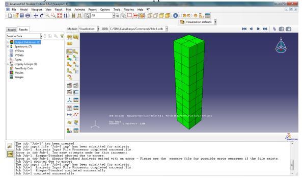
To view the deformed shape with stress contours, click the Plot Contours on Deformed Shape button on the toolbar.
