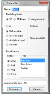
We will make a rectangular extrusion. Click the rectangle in the sketch tools. In the dialog box at the bottom of the window, type 0,0 for the starting corner of the rectangle. Press Enter. Type 0.2,1 for the opposite corner of the part and press Enter.
