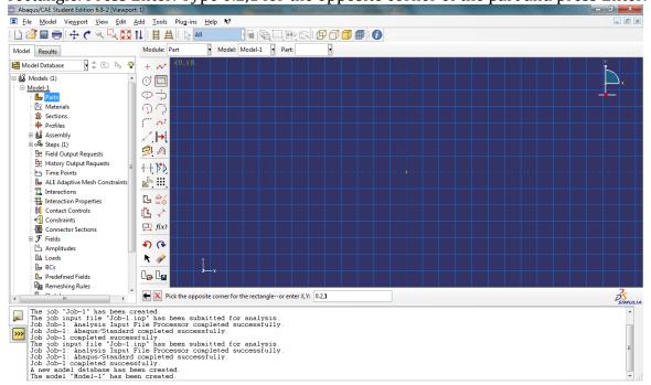
Click on the X button. Fill out the desired depth for the extrusion. In this case we will give the bar a square cross-sectional area so choose 0.2. Press Enter. A rectangular bar should now appear in the ABAQUS CAE window.
