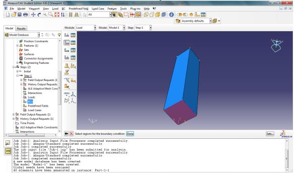
In the Edit Boundary Conditions window that appears, check the boxes for U1,U2 and U3, and enter a value for displacement of 0 for all. Click OK.
