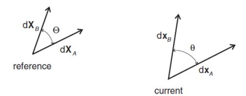
Calculate angle after deformation:
