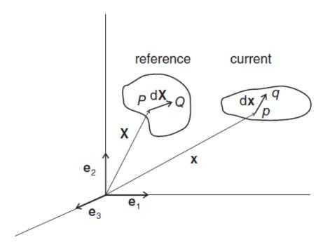
Definition of deformation gradient tensor:
