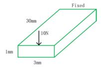
The dimension of the part is shown above and we apply a force, 10N, on one end, while the other end is fixed. Now, we will use Abaqus to solve this problem. We assume this part is made by a kind of steel with Young's Modulus, 209000*MPa*, and Poisson ratio 0.269.
