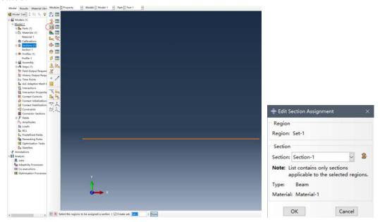
Assign the beam section oritation in the assign menu. Then select the line and click done. Define the direction as default.
