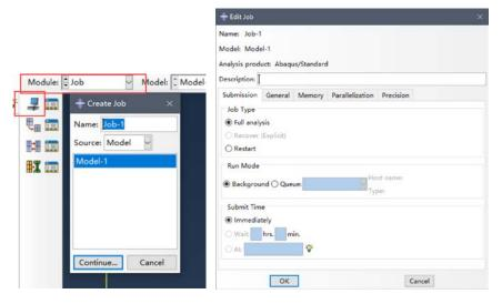
Then, open the 'Job Manager', and submit the job to solver. The processing information is shown in the bottom.
