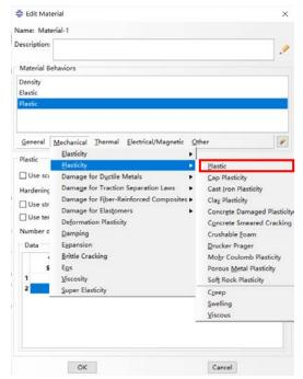
Then click the drop-down icon besides *Hardening* option. For linear isotropic plasticity, choose Isotropic in the list; while pick hardening for linear kinematic plasticity.
