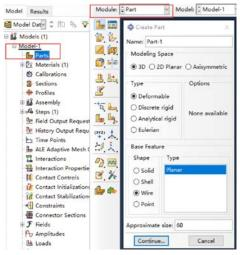
Next, choose command 'Line', and then input the two coordinate of the line, (0,0) and (30,0) in the bottom, prompt box. And follow the instruction in the bottom to finish the part.
