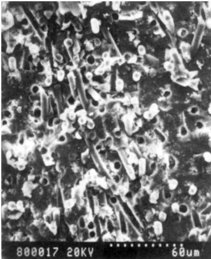
Carbon fiber reinforced ceramic composite fracture surface
