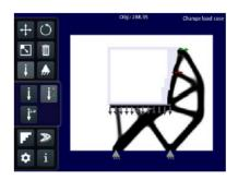
Example 2: Effect of making each load a separate load case.
