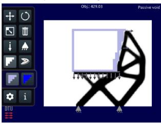
**Example 1:** The chair design is constructed using a single load case with the following settings: The downward "seat" load is 2.0 times larges than the two right oriented point loads. The volume fraction is set to 0.16 and an passive void domain is included to keep the seat free of material.
