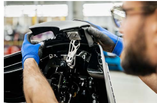
BMW i8 soft-top attachment component is 3D printed with aluminum
