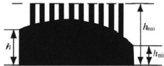
Cross-section of the upper half of a rib-stiffened plate with one field of stiffeners running along the normal of the cutting plane.
