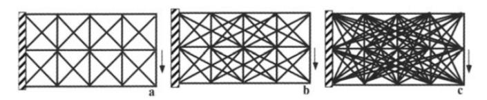
Ground structures for transmitting a vertical force to a vertical line of supports. Truss ground structures of variable complexity in a rectangular domain with a regular 5 by 3 nodal layout. In c) all the connections between the nodal points are included.
