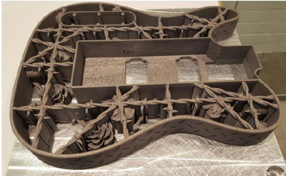
Aluminium guitar still welded to build plate after coming out of the printer, having the loose powder vacuumed away, and being heat treated
