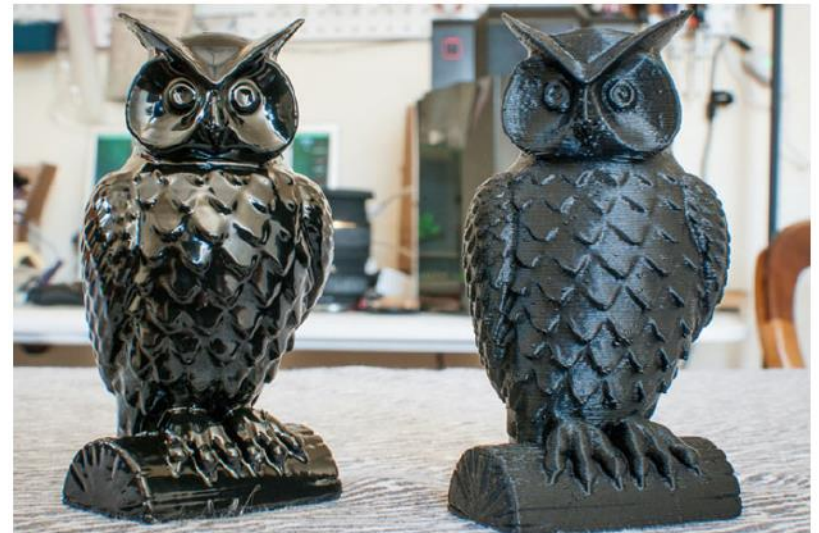
Acetone vapour smoothed ABS parts
