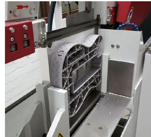
Aluminium guitar being cut off the build plate with a saw
