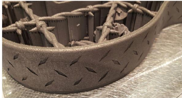
Support material that must be removed from aluminium guitar
