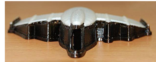
Part printed with soluble support material
