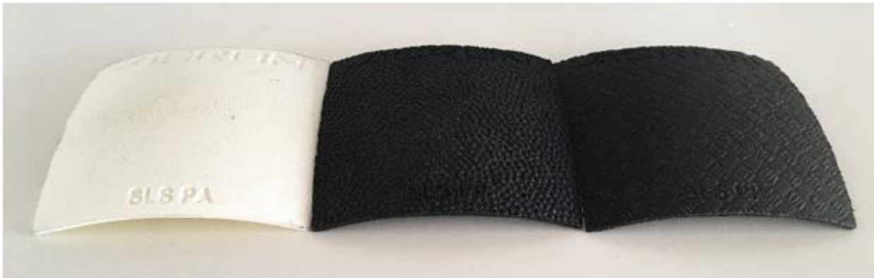
Texturing the curved surface of a part almost entirely eliminates the stair-step effect. The left part clearly shows stair-stepping, whereas the textured parts do not
