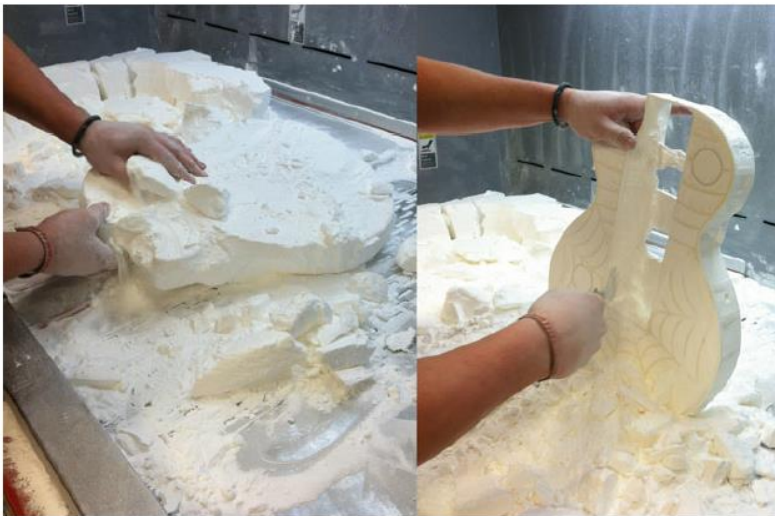
Powder bed fusion parts being removed from the powder 'cake' Part designed with cleanout holes to make depowdering of the part easier
