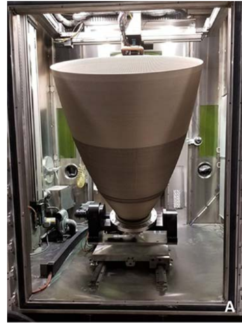
Examples of Large Scale DED at NASA. A) LP-DED integral channel nozzle 6000 (1.52 m) diameter and 7000 (1.78 m) height with NASA HR-1 alloy deposited in 90 days, B) Powerhead half shell using Inconel 718, and C) LP-DED JBK-75 Nozzle (no channels) that is 1/2 scale RS-25.
