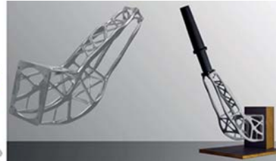
TO process of an antenna bracket for the Sentinel-1C and Sentinel-1D. Photo courtesy of Altair Engineering
