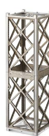
Test configuration of the bracket with adaptor plate and dummy masses. Copyright: The American Institute of Aeronautics and Astronautics (AIAA), Inc
