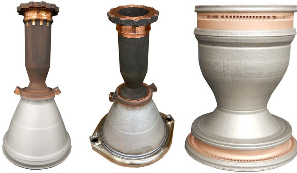
a: Bimetallic 7k Coupled Chamber using L-PBF GRCo-42 with HR-1 DED Integrated Nozzle (b: complete with manifolds). c: Bimetallic 40k Chamber built using L-PBF GRCo-42 liner and HR-1 DED Jacket. (Courtesy: NASA)
