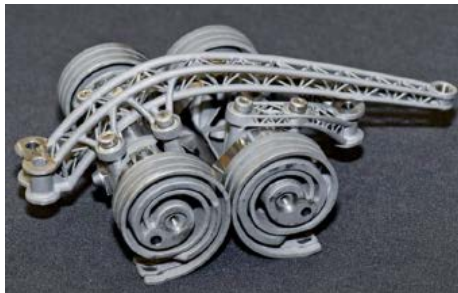
Example of 1.5 m mirror support being manufactured as technology demonstrator (image courtesy of Fraunhofer and European Space Agency)
