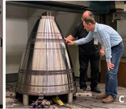
Examples of Large Scale DED at NASA. A) LP-DED integral channel nozzle 6000 (1.52 m) diameter and 7000 (1.78 m) height with NASA HR-1 alloy deposited in 90 days, B) Powerhead half shell using Inconel 718, and C) LP-DED JBK-75 Nozzle (no channels) that is 1/2 scale RS-25.
