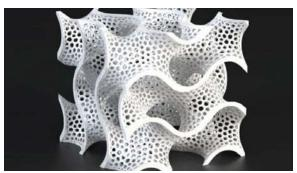
Use a mix of virgin powder and used powder. Typically, the ratio of new to old powder ranges from 20/80 to 35/65.
