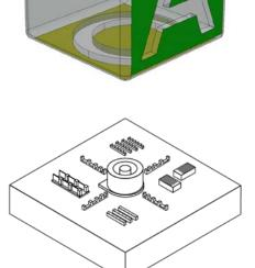
ISO/ASTM 52902:2019 Additive manufacturing — Test artifacts — Geometric capability assessment of additive manufacturing systems
