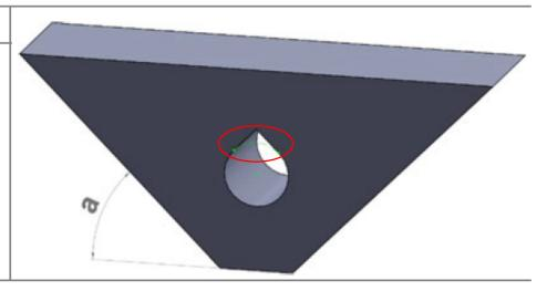
Horizontal holes (e.g., cooling channel profiles) can often be modified into teardrop or ovals shapes to minimize the need for internal supports that are hard to remove.
