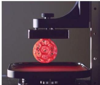
SLA is one of the few processes where the parts are relatively isotropic. This is because the layers chemically bond to one another as they print, resulting in near identical physical properties in the X, Y, and Z-direction.
