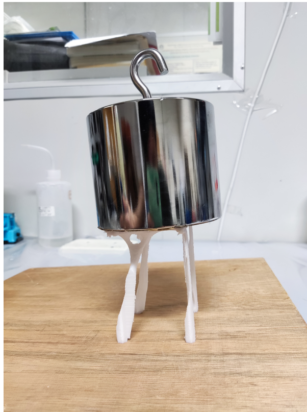
Figure 3: Printed parts with 5 kg loads on it.
