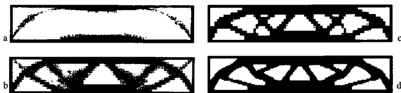
Fig. 3.6. Optimal design using a rank-2 material strain energy density with penalties on intermediate densities and on perimeter. a) shows the density distribution for the unpenalized case. In b) intermediate densities are penalized. In c) and d) intermediate densities and perimeter are penalized, with d) being a fine mesh variant of c) (from Jog et al. 1994).
