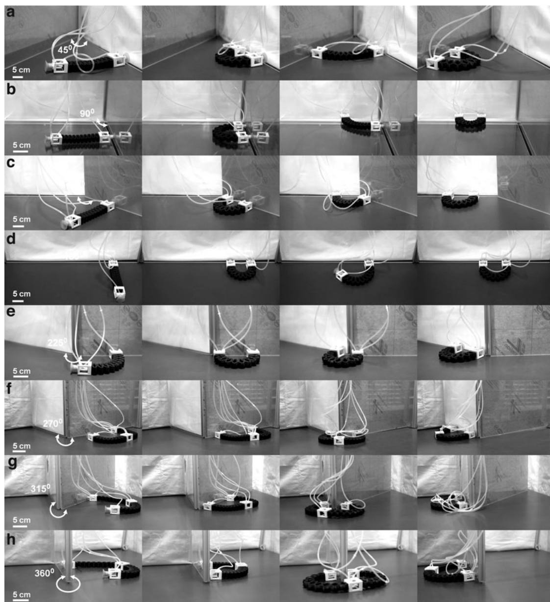
FIG. 10. The soft robot with flipping locomotion based on one or two KiriSPAs for transition between two surfaces: (a) 45°; (b) 90°; (c) 135°; (d) 180°; (e) 225°; (f) 270°; (g) 315°; and (h) 360°.
