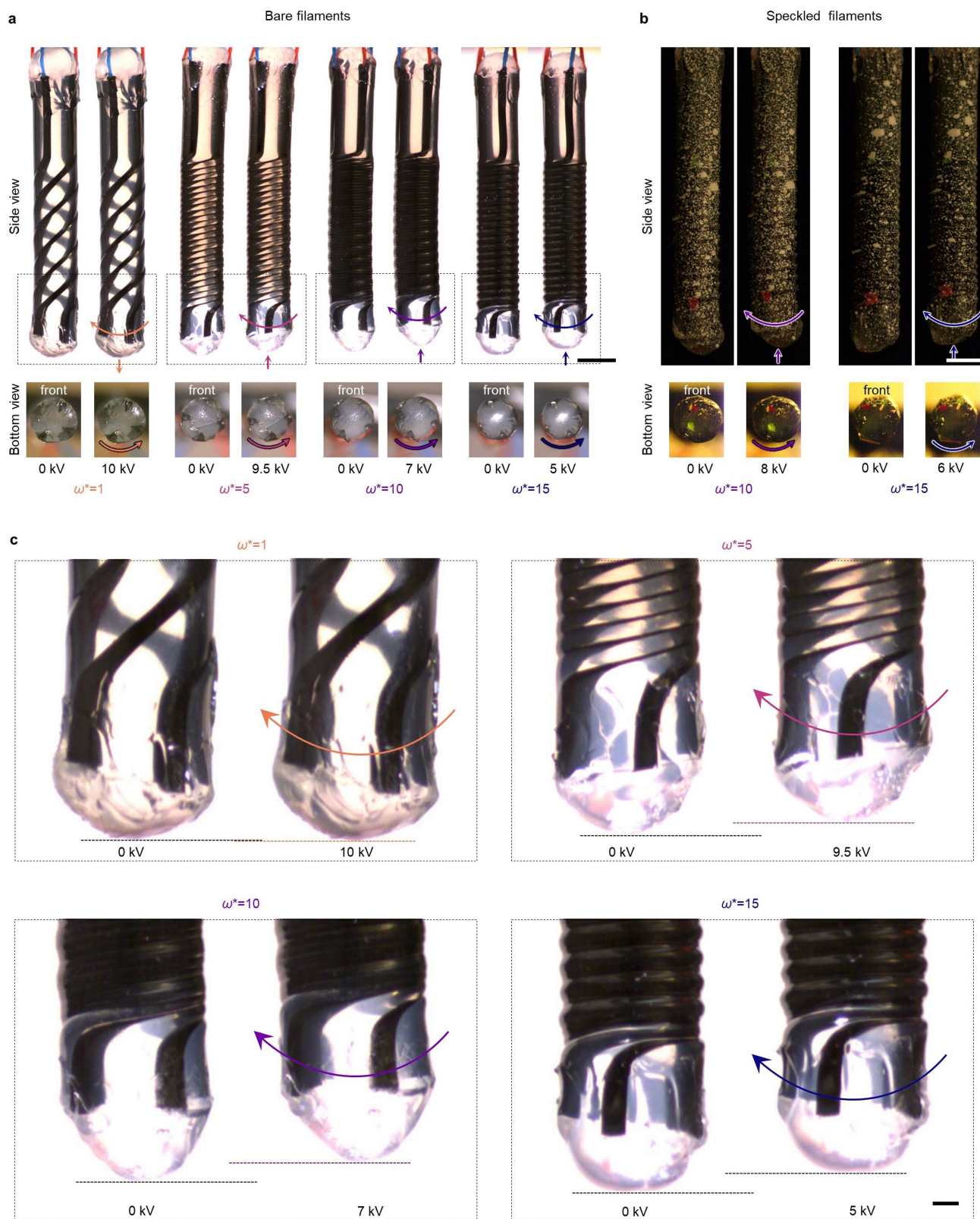
Extended Data Fig. 7 | Actuation of HDEAs printed in the vertical configuration ( \theta_p = 90^\circ , \theta_d = 90^\circ ). Photographs of side views and bottom views of several HDEAs before actuation (0 kV) and during actuation (>0 kV), showing filament twisting and axial extension ( \omega^* = 1 ) or contraction ( \omega^* = 5, 10 and 15).
