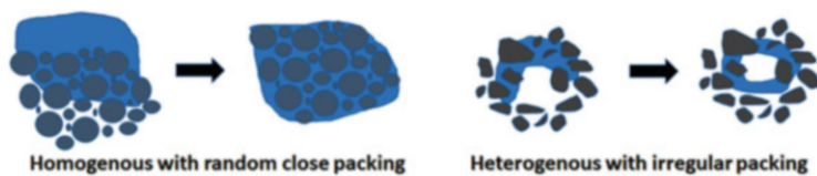
Fig. 7.8 Schematic presentation of binder penetration within homogeneously and heterogeneously distributed powder beds
